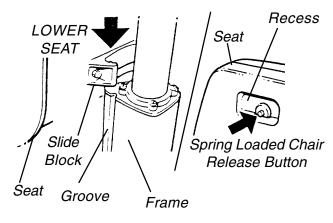
FIGURE 10 - INSTALLING THE SEAT
